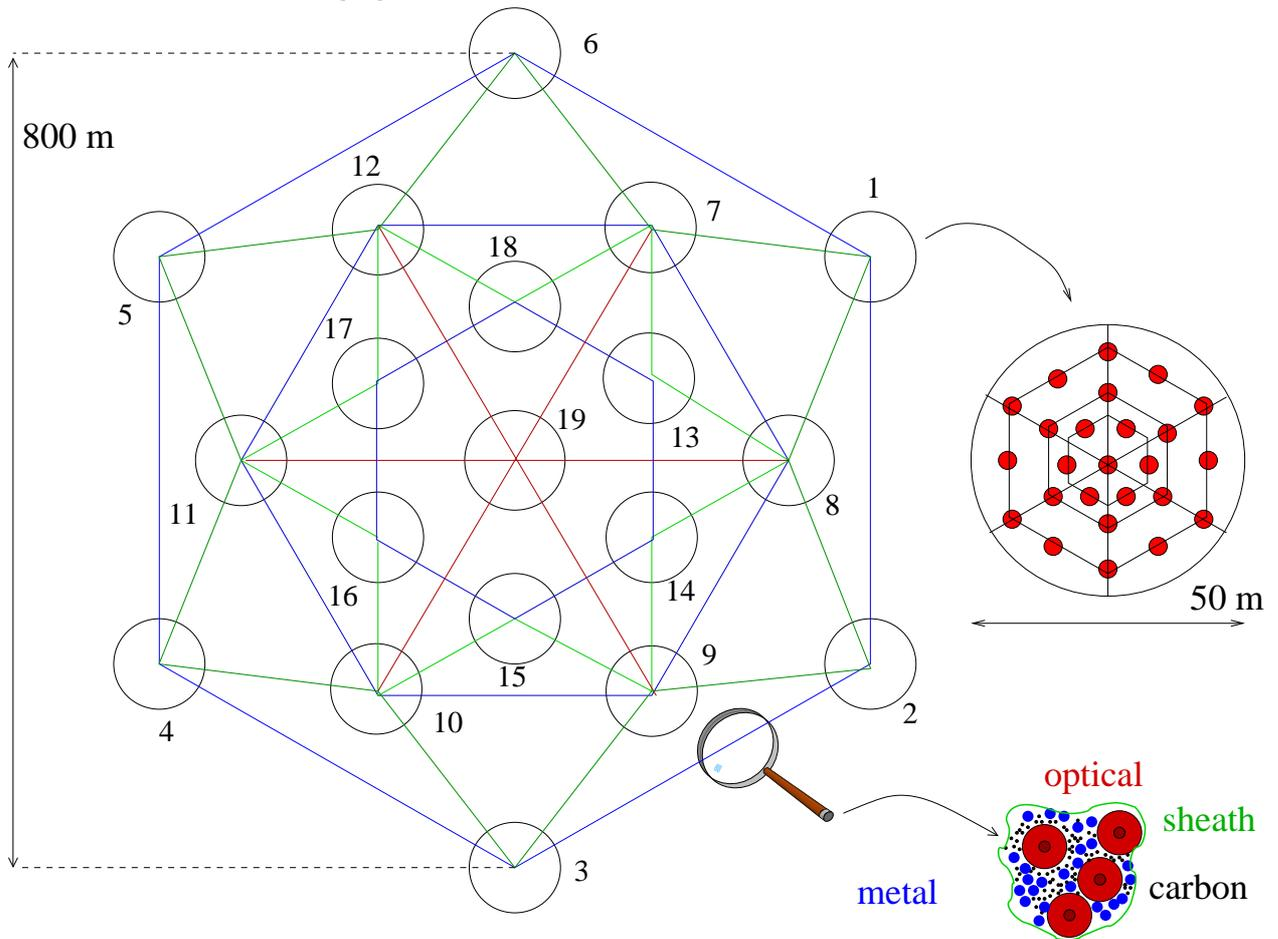
Figure 4: Left: The large web connecting 19 nodes by optical fibers and thin electrical wires. Right: One node containing 25 transponders, connected to each other by optical fibers and thin metal wires attached to a thin Mylar foil. As shown, the total length of wire connecting the nodes is 11.4 km. Lower right: cross section of a wire with carbon fibers, optical fibers, and metal filaments.
