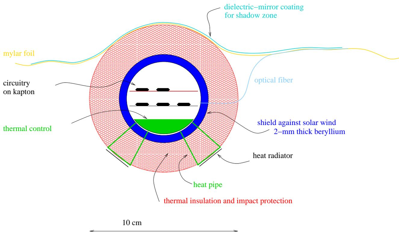
Figure 13: Schematic cut through a transponder, see also fig. 7. The electronics are inside a beryllium shell that protects against lower-energy solar protons (sec. 5.7). A thermal-control unit contains heaters and thermoelectric coolers, and dissipates heat through heat pipes leading to radiators that are in the shadow (see text). The central transponder of each node is slightly larger to hold the electronics for power sharing and communication with the other nodes, as well as the atomic clock.
