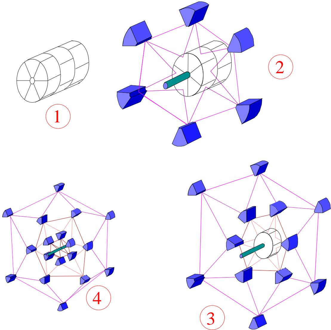
Figure 5: Deployment of the coarse web. A space vehicle (1) carries the array to the asteroid. It is comprised of three sections, each containing six slices. These are ejected in sequence (2-3-4) to deploy the web. After ejection of all slices, the entire web is made to rotate slowly to keep it stretched out (see text). Finally, each of the slices deploys a sub-web, as shown in fig. 6.
