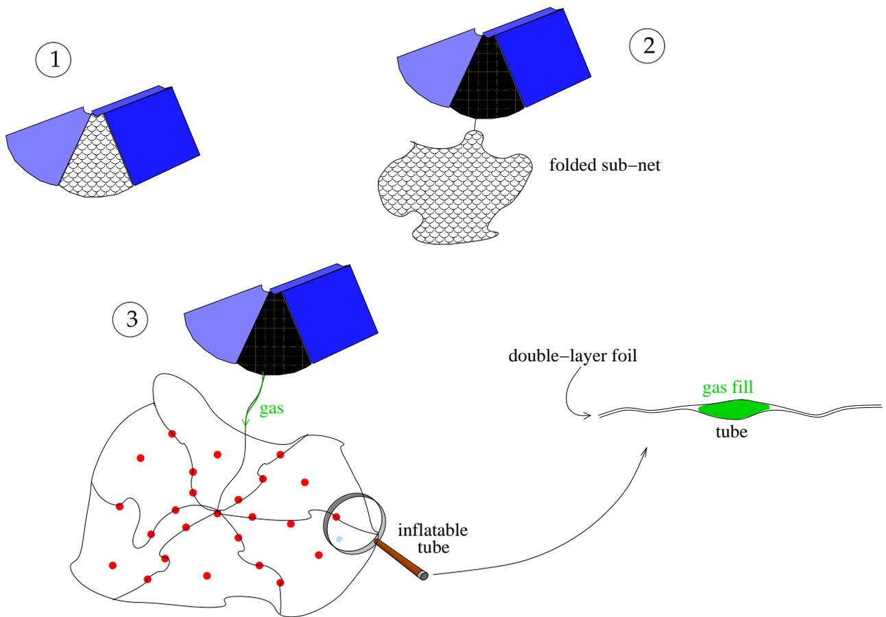
Figure 6: Ejection and unfolding of the sub-webs: 1: container opens, 2: folded Mylar foil is ejected, 3: foil unfolds as gas is blown into tubes formed between two layers of the foil.
