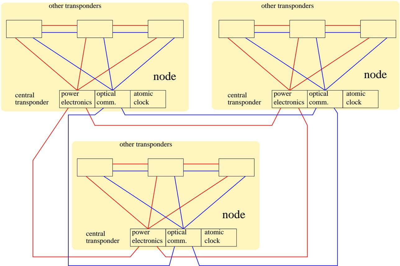
Figure 10: Schematic of the array showing 3 of the 19 nodes, each with the central transponder (see fig. 7) communicating (blue) and sharing power (red) with other transponders of the node, as well as communicating and sharing power with other nodes.
