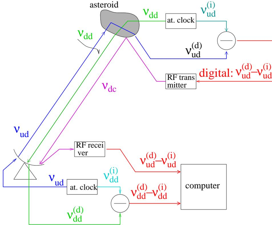
Figure 3: Modified coherent link: Frequencies derived from free-running atomic clocks on the ground and on the asteroid are transmitted, and are compared on both sides. The phase slippage measured on the asteroid is transmitted to the ground for comparison with the one measured there.
