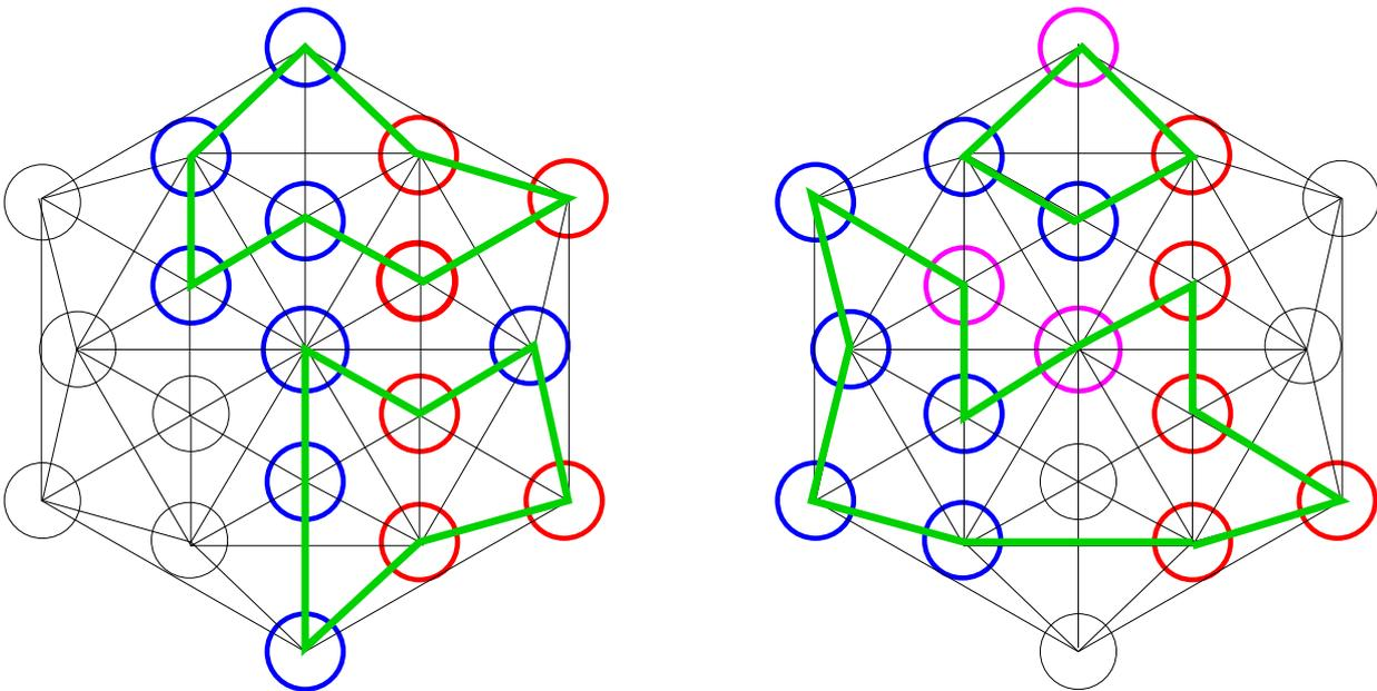
Figure 9: The power-distribution scheme. Current paths are switched rapidly between different configurations, each containing some nodes acting as electric power sources, some as power consumers, and possibly some “spectators”. Two possible configurations are shown here with sources in red, consumers in blue, spectators in magenta, and active current paths in green.
