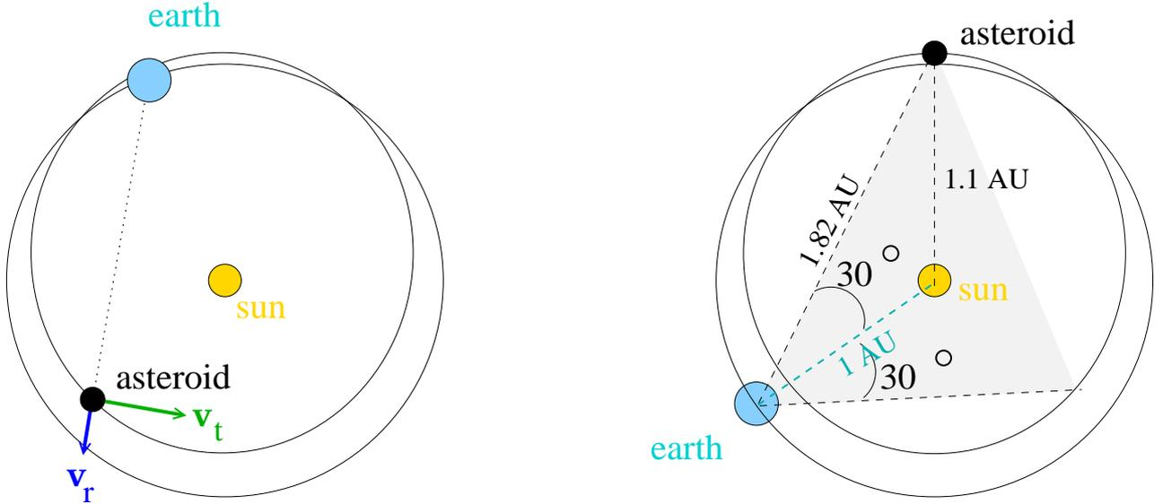
Figure 1: The design goals are a Doppler accuracy of  $10^{-6}$  m/s for the radial velocity  $\mathbf{v}_r$  and a ranging accuracy of 5 m for most of the asteroid's orbit, except for an angle of  $\pm 30^\circ$  from opposition to the earth (the shaded area, see also fig. 15). The maximum earth-to-asteroid distance is 1.82 A.U.
