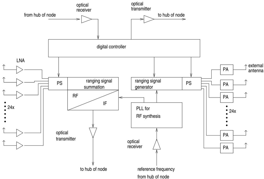
Figure 12: Radiofrequency circuitry for ranging inside each transponder. “PS” means multiple (24x) phase shifters, “LNA” means low-noise amplifier, and “PA” means power amplifier. The Doppler and communications circuits are similar.
