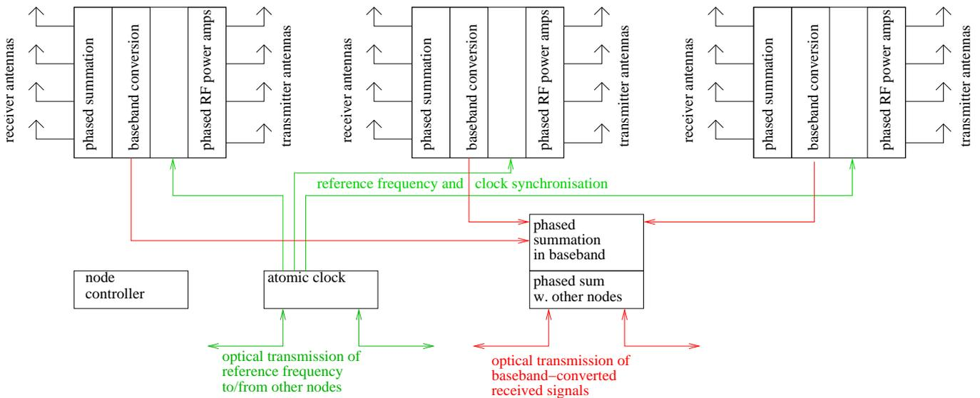
Figure 11: Node electronics showing three of 25 transponders, each with multiple antennas for reception and transmission. The nodes distribute the received and baseband-converted signals across the web for decentralized data processing, and any one node may be providing the reference frequency.
