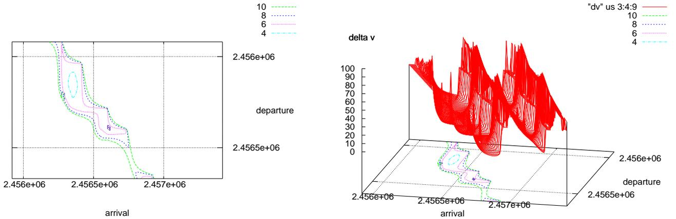
Figure 14: Arrival vs. departure dates for total velocity changes  $\Delta v_d + \Delta v_a = 4, 6, 8, 10$  km/s for departure from earth after LEO breakout, and rendezvous with Apophis. Minimum  $\Delta v$  for departure on epoch 2456132 (2012/7/23), arrival on epoch 2456345 (2013/2/20), see fig. 16. Program available at [55], similar plots in ref. [57].
