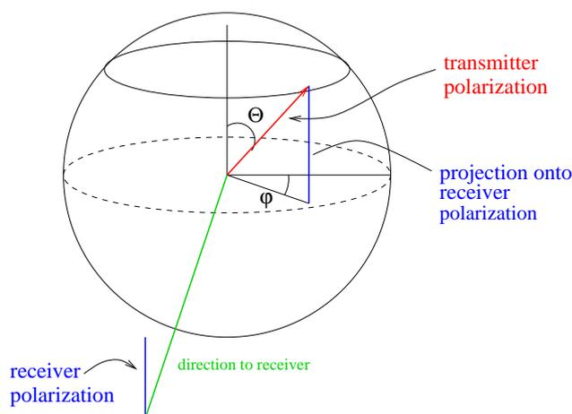
Figure 18: Sphere representing uniform distribution of random dipole orientations.
